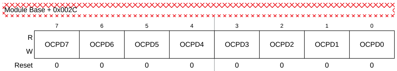
Figure 14-28. Output Compare Pin Disconnect Register (OCPD)
