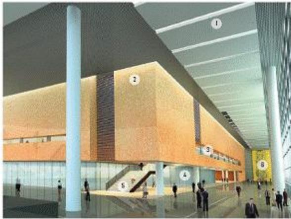
The upper level of the Plenary Hall continues the lighting language found below. Linear ceiling lighting elements identify the main public space. The form of the hall is grazed with light from a slot which defines the perimeter of the core. Long apertures carved into the core walls allow views through to illuminated corridors. Uplight on the massive wood ceiling and luminous stair risers lead visitors to the upper levels.
