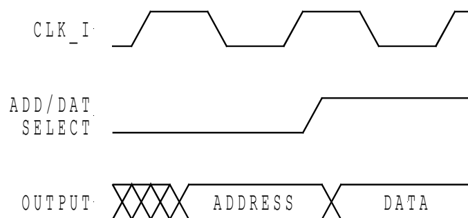
Illustration 8-17: Circuit and timing diagram for a multiplexed address/data bus
