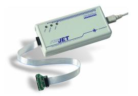
JTAGjet™ is a small, universal In-Circuit Debugger that connects to targets via the JTAG port. It is equipped with USB 2.0 high-speed port and on-board FPGA to achieve download speeds of up to 2MBytes/sec. JTAGjet-Trace™ has the same features as JTAGjet but contains ETM and PTM real-time trace capture logic with up to 18 MBytes of memory.
